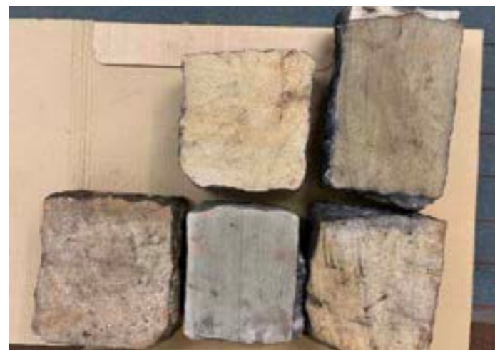
SAWN COBBLES EXPOSE THE RANGE OF COLOUR VARIATION PRESENT ON-SITE
