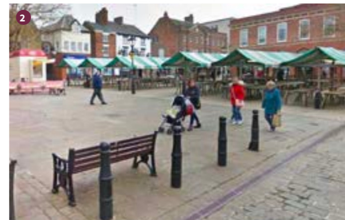
2 BOLLARDS AND SEATING PROVIDE HVM TO THE WESTERN ONLY SIDE OF NEW SQUARE
